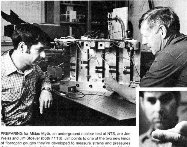
Weiss and Jim Stoever (both 7116). Jim points to one of the two new kinds of fiberoptic gauges they've developed to measure strains and pressures during weapons tests. In the close-up view at right, Joh holds one of the Ushaped fibers that can be used as either a pressure gauge or a strain
